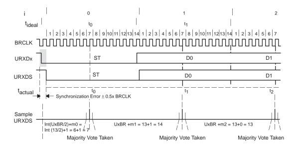
The ideal start bit timing  $t_{ideal(0)}$  is half the baud-rate timing  $t_{baud\,rate}$  because the bit is tested in the middle of its period. The ideal baud rate timing  $t_{ideal(i)}$  for the remaining character bits is the baud rate timing  $t_{baud\,rate}$ . The individual bit errors can be calculated by:
